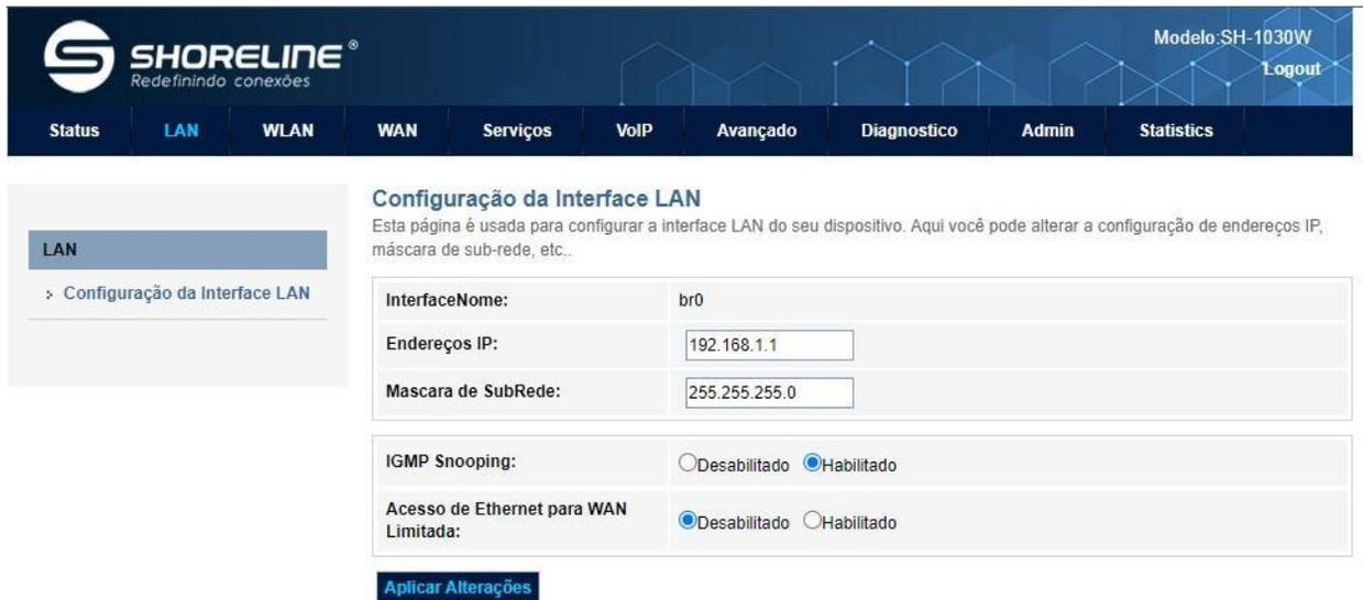
The screenshot shows the Shoreline web interface. At the top, there is a navigation bar with tabs: Status, LAN, WLAN, WAN, Serviços, VoIP, Avançado, Diagnostico, Admin, and Statistics. The 'LAN' tab is selected. Below the navigation bar, the page title is 'Configuração da Interface LAN'. A sidebar on the left shows a tree view with 'LAN' expanded and 'Configuração da Interface LAN' selected. The main content area contains the following configuration fields:
